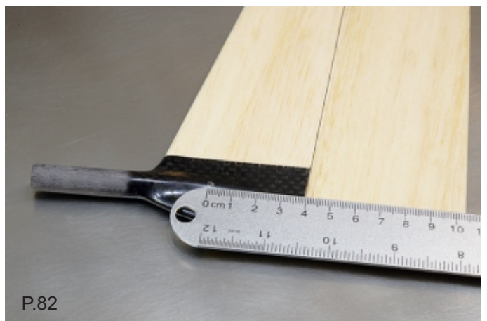
25. Hold boom with elevator tube pointing UP then position stabilizer mount on the top with front of the mount aligned with masking tape edge and, using pencil outline its position. PHOTO 79
