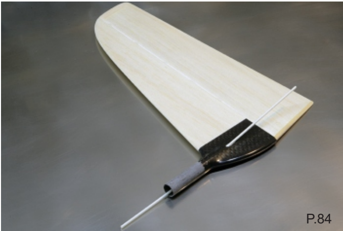
30. Now holding rudder push-rod wire projecting from boom end insert it into tube projecting from stabilizer tip then push stabilizer until stabilizer tip fits inside the boom. PHOTO 85 & 86
