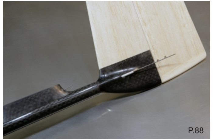
32. Aligning with push-rod wire mark position for the rudder control horn, drill two small holes in the rudder for the horn mounting posts. Then trial fit control horn and check alignment. PHOTO 88 & 89
