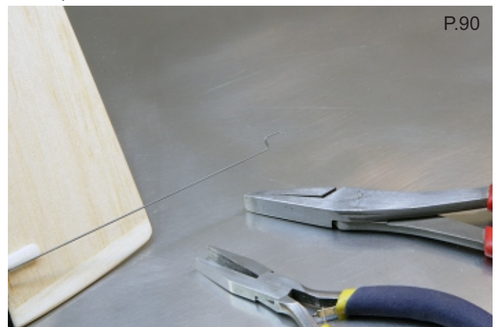
34. Take rudder control horn and connect to the "Z" bend. Then deflecting rudder to the right push control horn post into rudder holes. PHOTO 91 & 92
